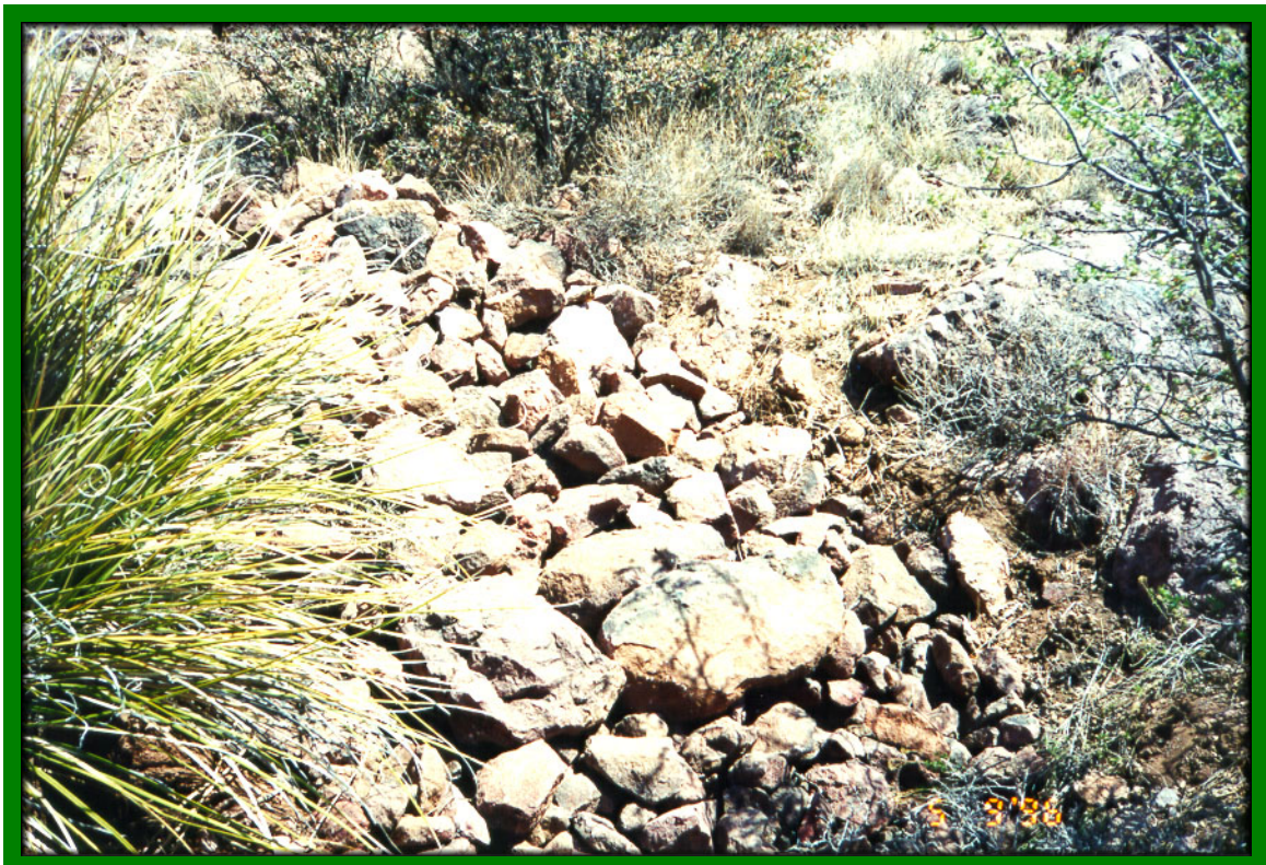
Feature 19 Adit backfilled with rock
