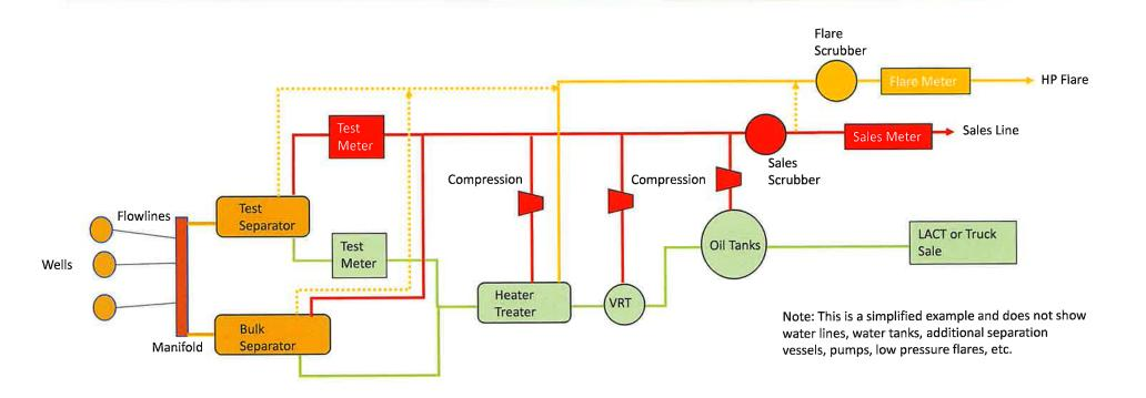
Most convenient flare meter location is on aggregated flare line, after any potential liquid removal
