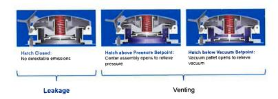
• Example 4: Fugitive emissions components: Fugitive emissions components emit gas to the atmosphere under normal operation and are authorized by NMED.
