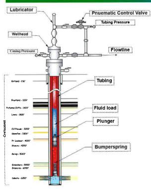
Figure 3: Plunger Lift Configuration
