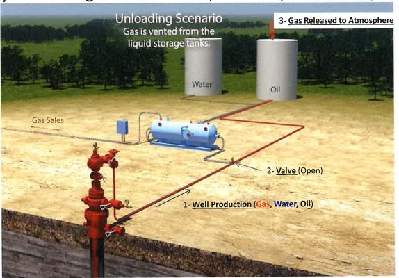
Figure 6: Unloading Scenario<sup>3</sup>
