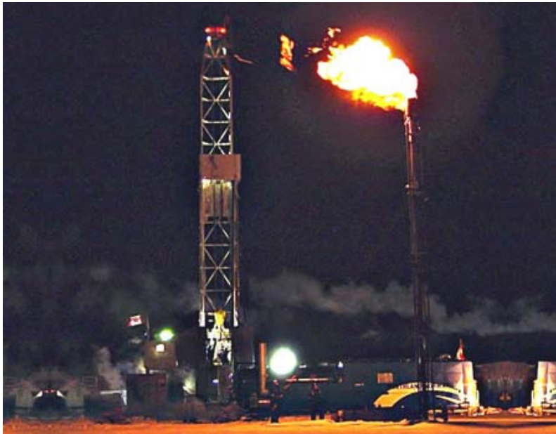
FIGURE 1. Photograph of the gas flare from the thermal gas hydrate production test in the Mallik 5L-38 Gas Hydrate Research Well. Photo with permission from S. R. Dallimore, Geological Survey of Canada. (Source) 1
