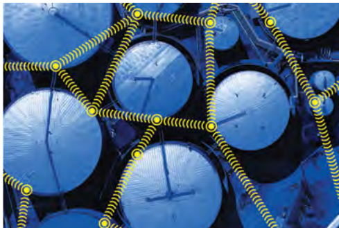
Figure 9.7: A self-organizing mesh field network can automatically find the best way around any fixed or temporary obstacles.
