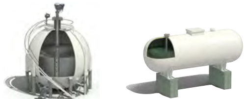
Figure 7.3: Spherical and horizontal tanks used for storing LPG.
