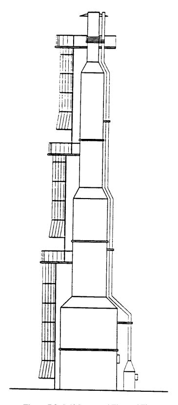
Figure 7.3: Self-Supported Elevated Flare
