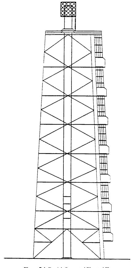
Figure 7.4: Derrick-Supported Elevated Flare
