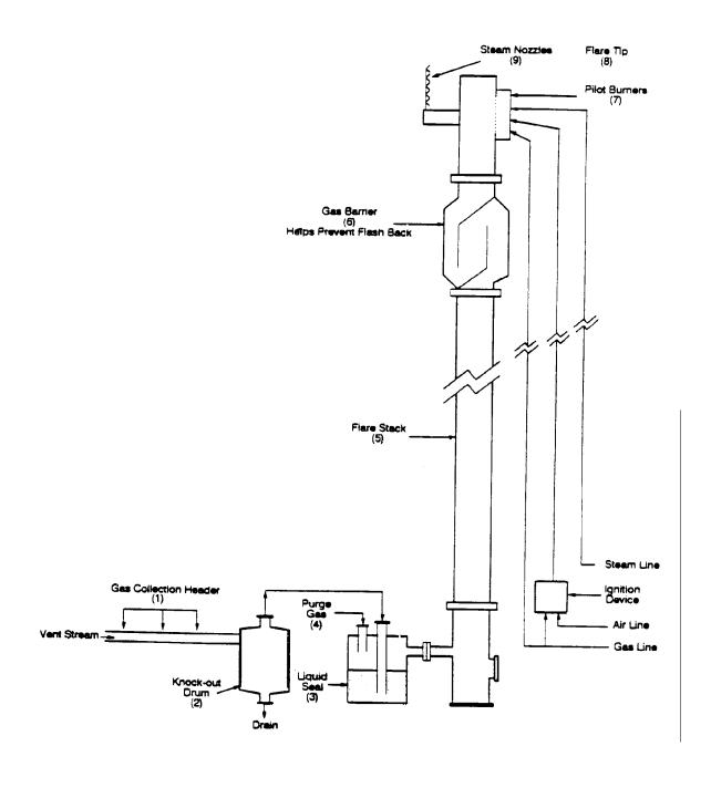
Figure 7.1: Steam-Assisted Elevated Flare System
