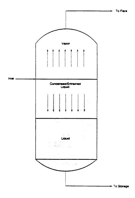
Figure 7.2: Typical Vertical Knock-out Drum
