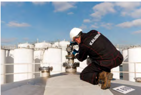
Figure 2.2: Hand gauging with a dipping tape.
