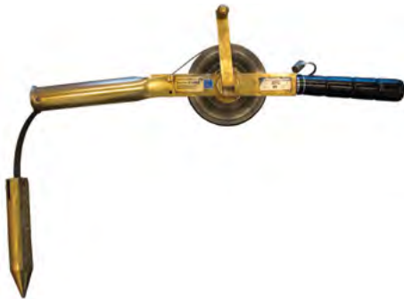
Figure 2.1: Hand dipping tape.
