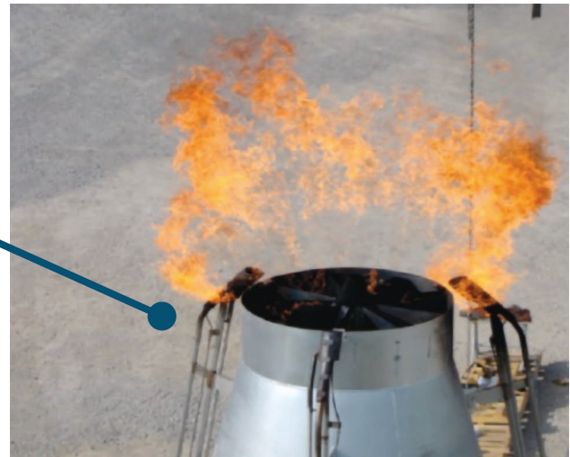
Figure 7b: An air-assisted flare with multiple wedge-shaped flow sections, alternating between air flow and gas flow
