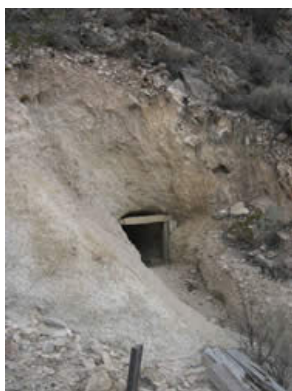
A mine adit leading to the inner workings in the mountain.
